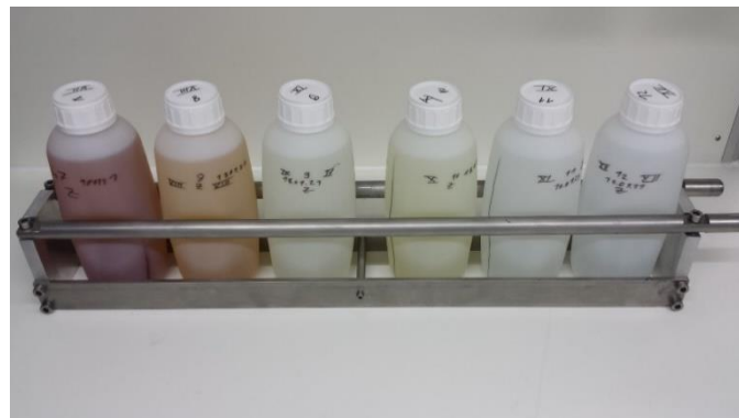
Fig. 2: Deformation device with PE-HD test bottles
