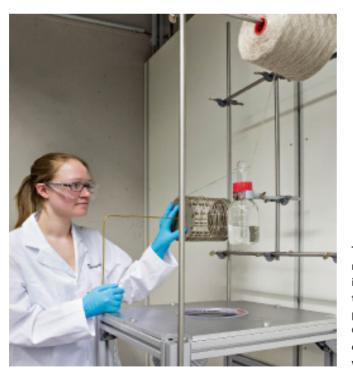
To make the natural fibers more resistant, the roving is impregnated with monomers: the polymerization then proceeds within the yarn. © Fraunhofer LBF | Picture in color and printing quality: www.fraunhofer.de/en/press
